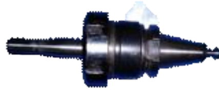
Figure (3) SPIF tool with tool holder
