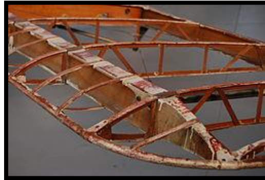
Fig - Wing ribs of a de Havilland DH.60 Moth
