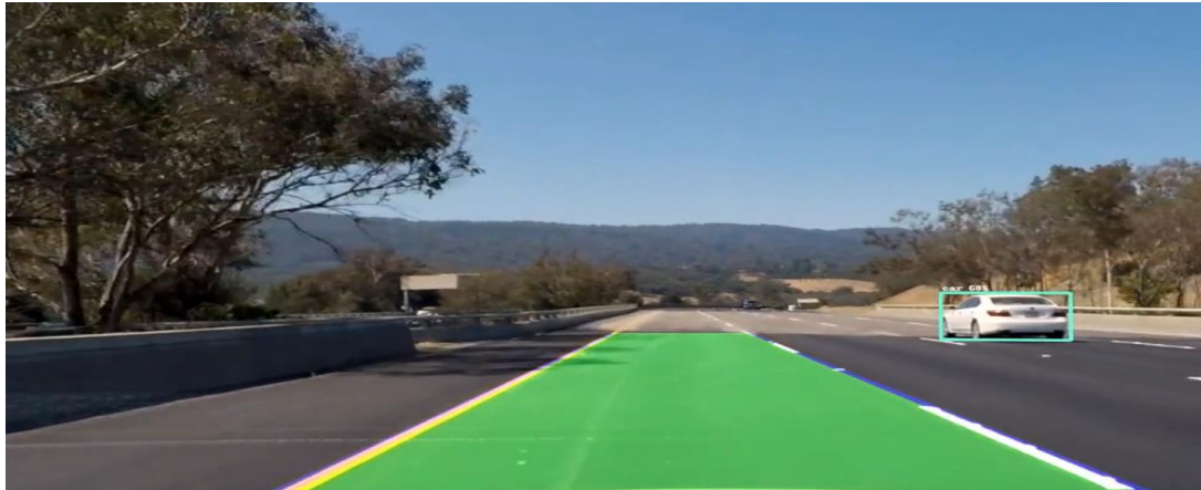
Fig 3.3 Output of the System with Lane bordering and anchor box on same side of road.
