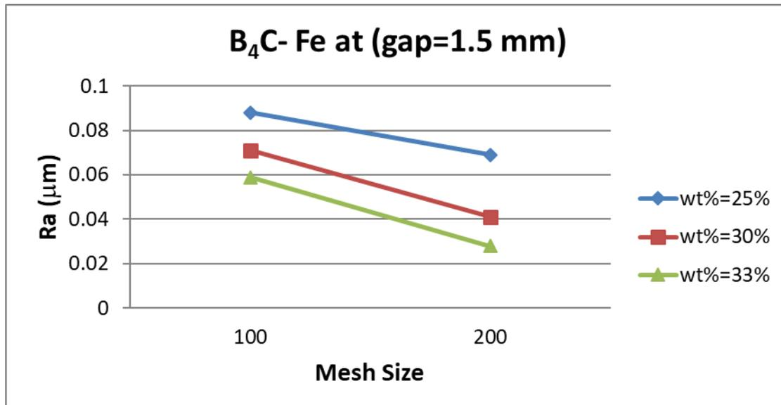
Fig (4) Effect of Mesh size and weight percent of B<sub>4</sub>C-Fe abrasive powder on Ra at gap=1.5 mm
