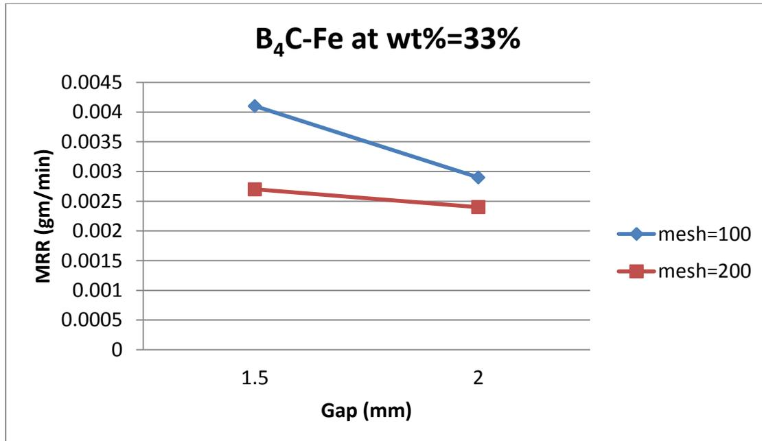
Fig (14) Effect of gap of B<sub>4</sub>C-Fe abrasive powder on MRR at wt%=33
