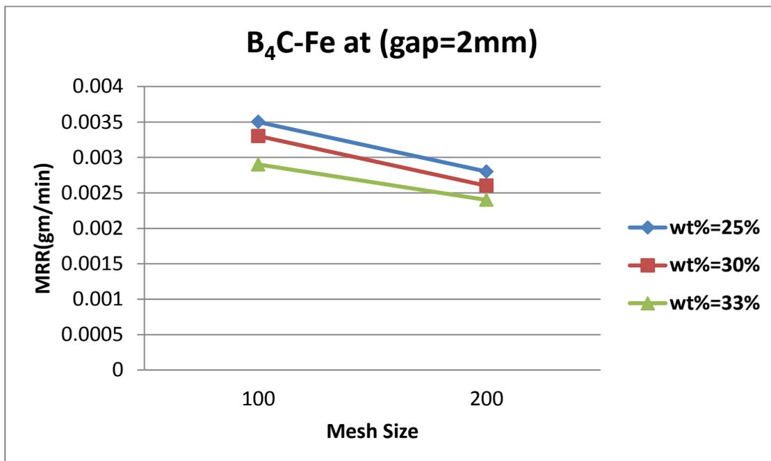
Fig (11) Effect of Mesh size and weight percent of  $B_4C$  -Fe abrasive powder on MRR at gap=2 mm
