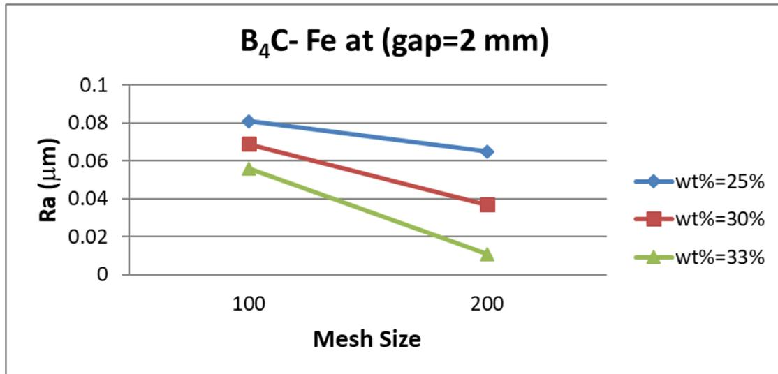
Fig (5) Effect of Mesh size and weight percent of B<sub>4</sub>C-Fe abrasive powder on Ra at gap=2mm
