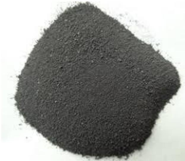
Figure (1) boron carbide
