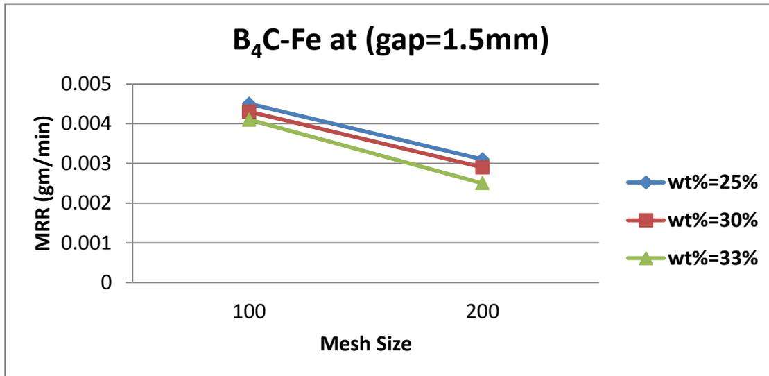
Fig (10) Effect of Mesh size and weight percent of B<sub>4</sub>C -Fe abrasive powder on MRR at gap=1.5 mm
