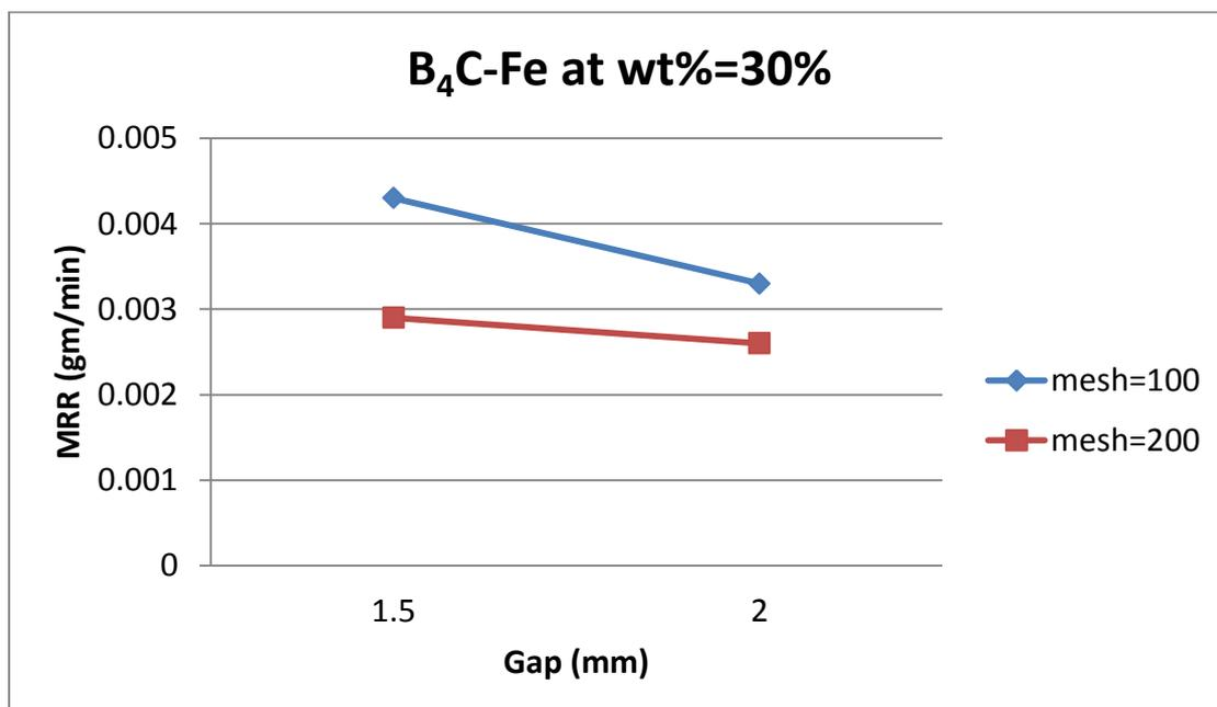
Fig (13) Effect of gap of B<sub>4</sub>C -Fe abrasive powder on MRR at wt%=30
