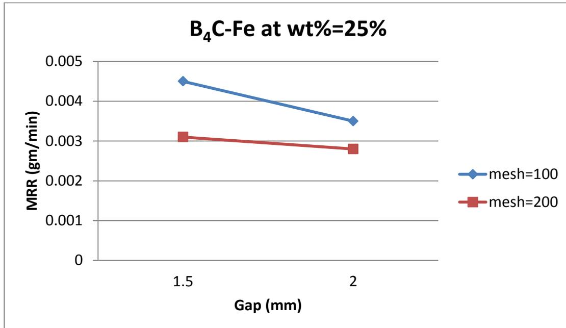
Fig (12) Effect of gap of  $B_4C$  -Fe abrasive powder on MRR at wt%=25
