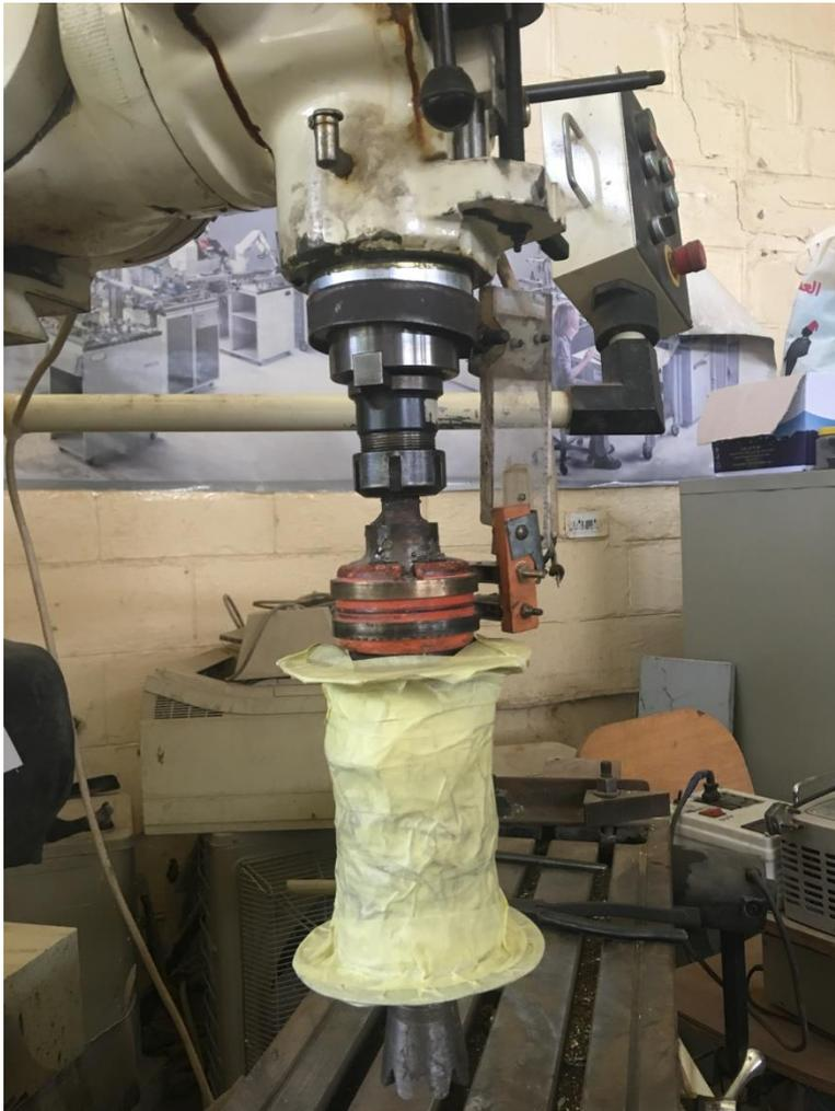
Figure (3) Magnetic abrasive machine
