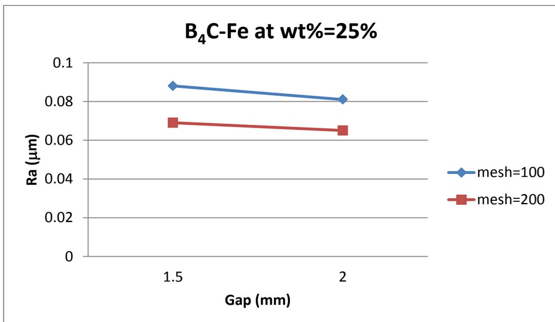
Fig (6): Effect of gap of B<sub>4</sub>C-Fe abrasive powder on Ra at wt%=25
