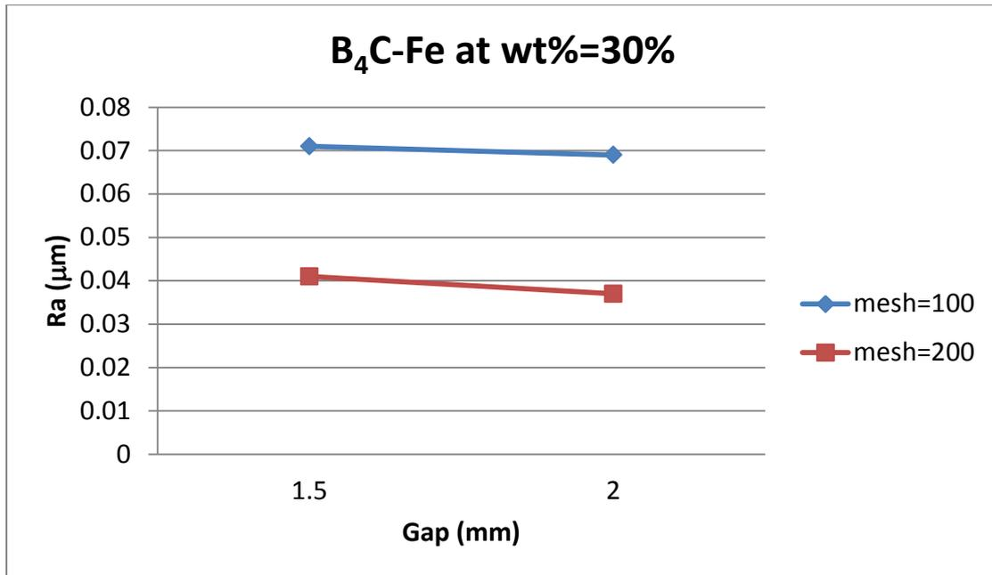
Fig (7): Effect of gap of B<sub>4</sub>C-Fe abrasive powder on Ra at wt%=30
