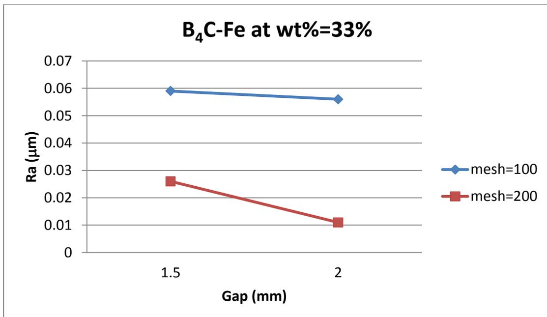
Fig (8) Effect of gap of B<sub>4</sub>C-Fe abrasive powder on Ra at wt%=33
