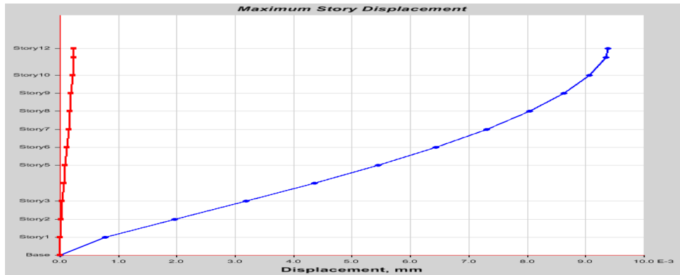
Fig.4.7.Displacement of Storey Response
