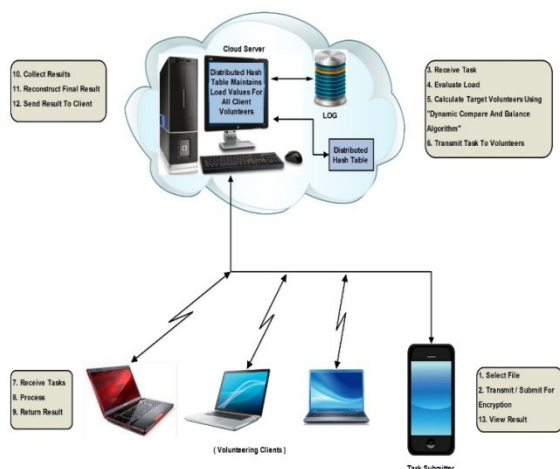
Figure 1. Block Diagram for Cloud based load balancing in ad-hoc network using dynamic compare and balance algorithm [13]
