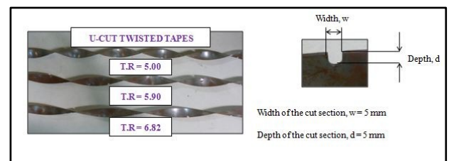
(c) U-Cut Twisted Tape (UTT)
