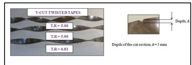
(b) V-Cut Twisted Tape (VTT)
