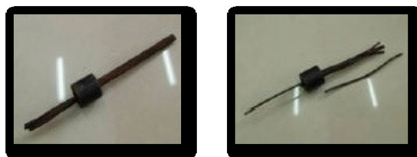
a) Virgin specimen b) Damaged strand specimen
