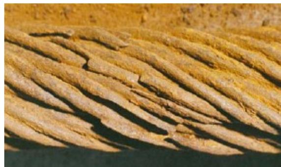
**Figure 3:** corrosion and break-up of 76 mm ungalvanized mooring rope after five years service
