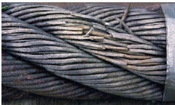
**Figure 6:** Damage caused where the tangent point was close to a crossover on a 70 mm mooring line after 8 years of service
