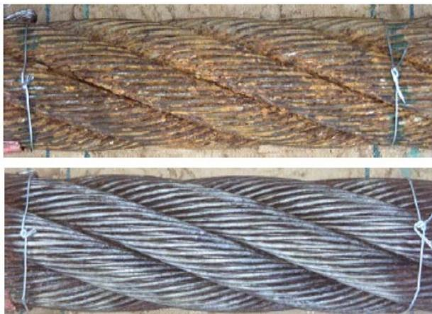
**Figure 2:** Effects of external corrosion on 90 mm Class B galvanized mooring rope
