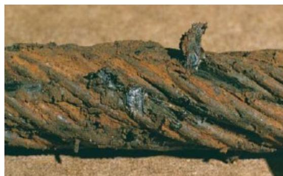
**Figure 4:** corrosion and break-up of 90 mm galvanized mooring rope after 7 years
