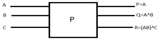
**Toffoli Gate**: Toffoli gate is a universal reversible gate which has three inputs (A, B, C) mapped to three outputs  $(P=A, Q=B, R=(A.B)^C)$ . The block diagram of Toffoli gate is shown in fig. 4:
