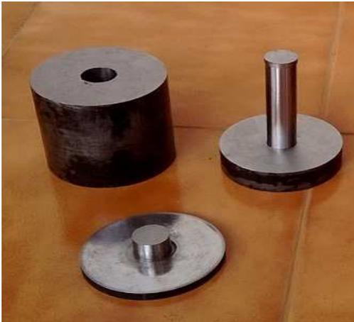
**Fig. 2:** Punch and die set according to ASTM B-925
