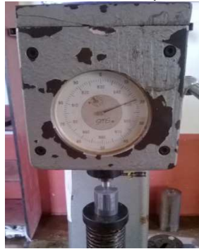
Figure 3. Rockwell hardness testing machine with test specimen
