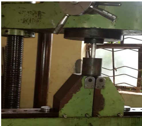
Figure 1. Compaction die set up kept in UTM.
