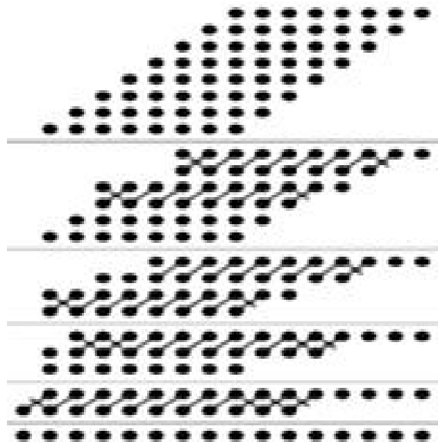
Fig.4. Method of Reduction on 8x8 Multiplier.
