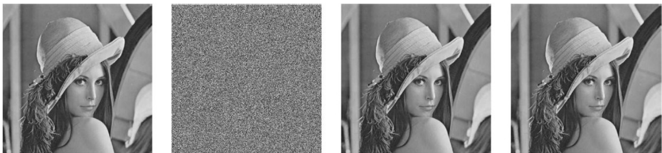
(a) (b) (c) (d) Fig.(a) Original image, (b) encrypted image, (c) decrypted image containing messages (embedding rate 0.1 bpp), (d) recovery version.
