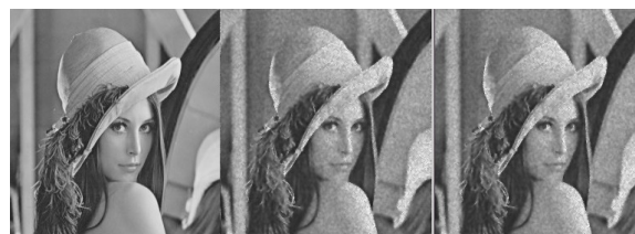
(a) Input image leena (b) Noisy image( \sigma=0.02 ) (c) Wiener filtered image.
