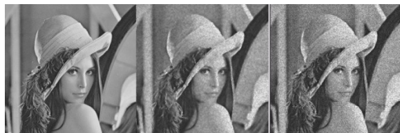
(a) Input image leena (b) Noisy image( \sigma=0.02 ) (c) DWT (level 4) filtered image.
