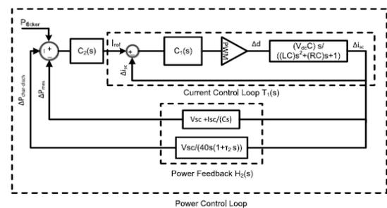
Fig.3. Small-signal block diagram for the super capacitor control loops.
