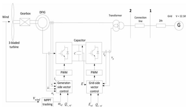
Fig1. Scheme of the DFIG-based wind turbine system
