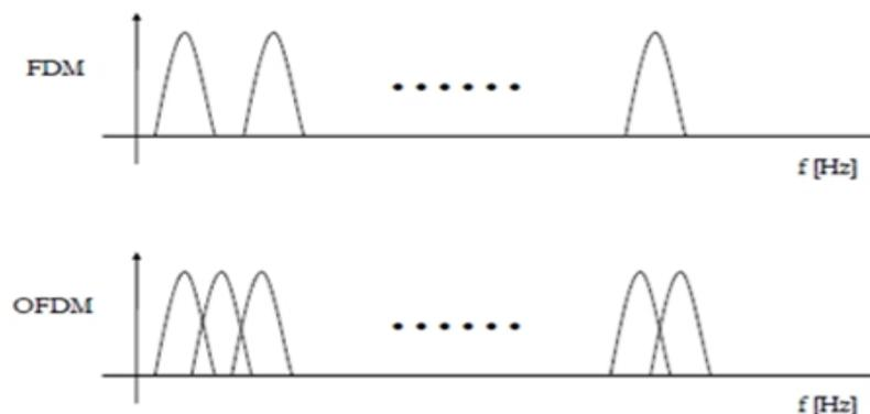
**Figure 2: Spectrums of FDM and OFDM**
