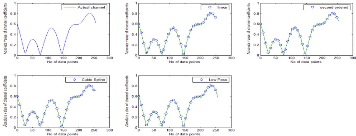
**Figure 6: Comparison of estimated channel coefficients for different interpolation techniques for MMSE estimate (5 PATH channel)**
