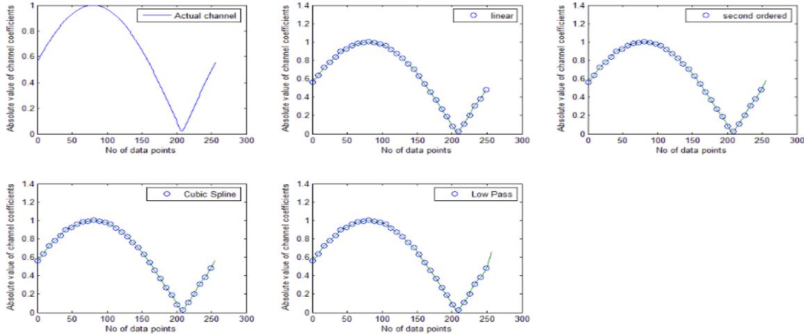
**Figure 5: Comparison of estimated channel coefficients for different interpolation techniques for MMSE estimate (3 PATH channel)**
