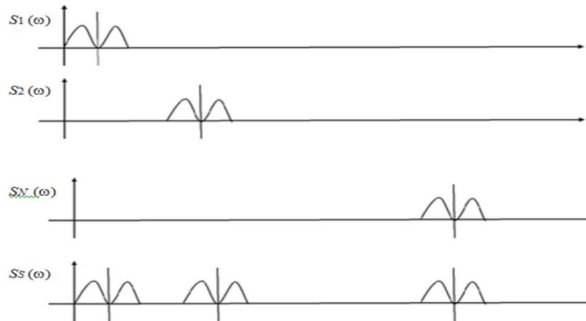
**Figure 1: Spectrum analysis of OFDM**
