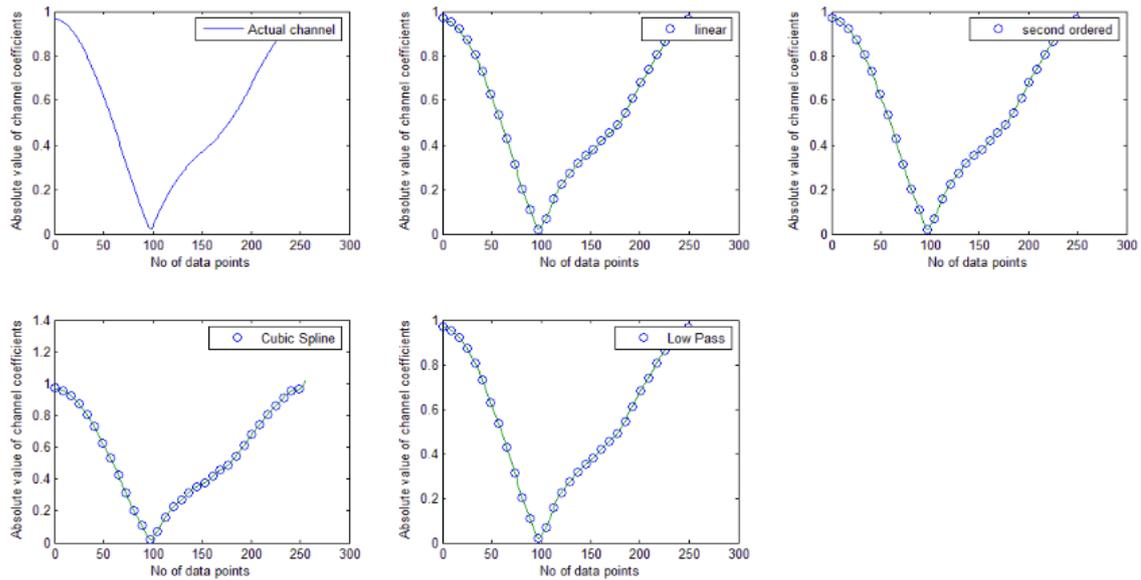
**Figure 3: Comparison of estimated channel coefficients for different interpolation techniques for Least Square Estimator (3 PATH channel)**
