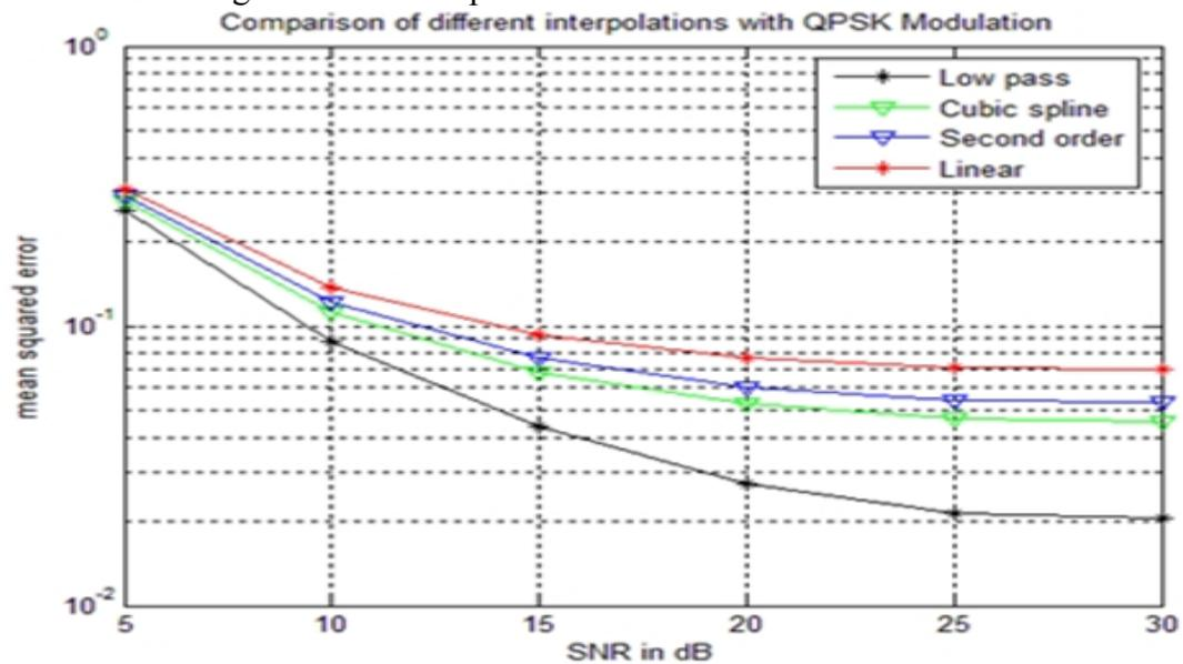
**Figure 7: Comparison of different interpolation schemes with QPSK interpolation:**
