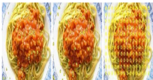
Fig. 2. Key point extraction techniques: (a) SIFT detector, (b) random sampling, and (c) dense sampling.
