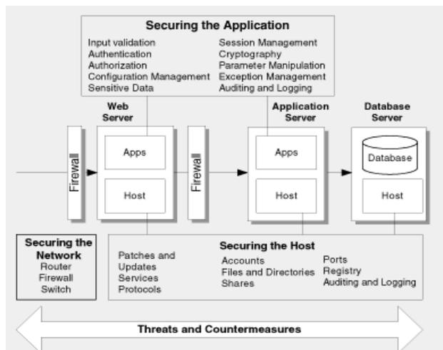
Figure 3: Securing network, host and application
