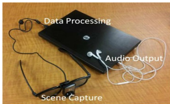
Fig. 3. Snapshot of our demo system, including three functional components for scene capture, data processing, and audio output.
