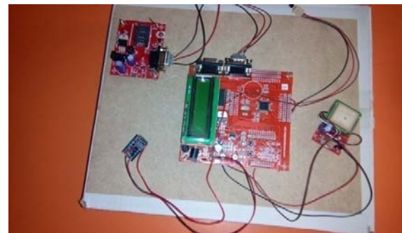
Fig 7: Vehicle monitoring system without power supply
