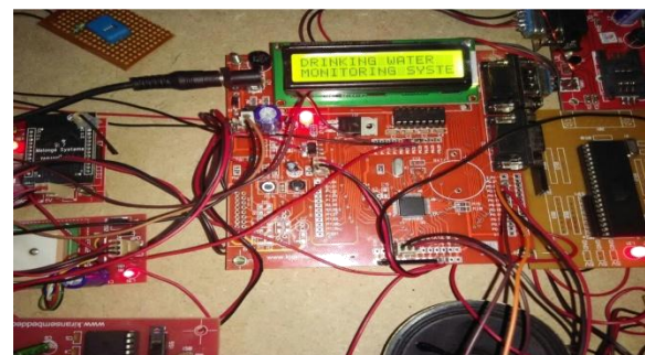
Figure2: Real time drinking water Quality monitoring and contamination detection system when power supply is connected
