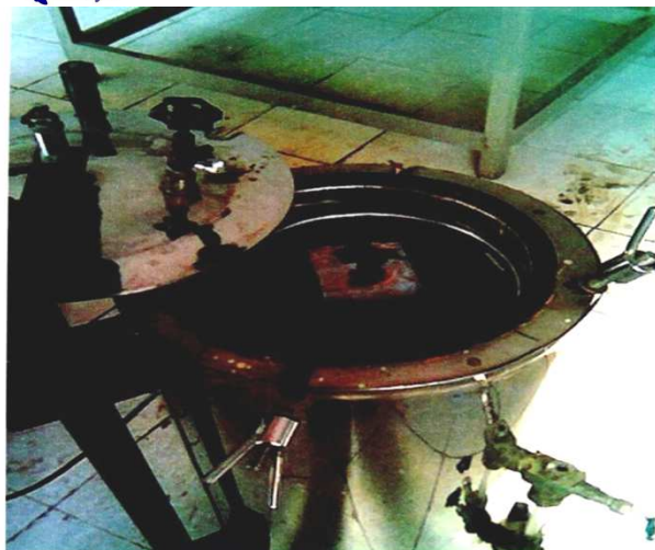
Figure-3 Autoclave Cube Testing at 90°C
