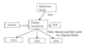
In Architecture Diagram clearly shows that the cluster head is chosen based on the LEACH algorithm. And each node is taking a part as a monitoring agent and also they can be act as a routing node. The cluster head is changed dynamically to avoid the redundancy in the path and also for to avoid the Hackers to track the path.
