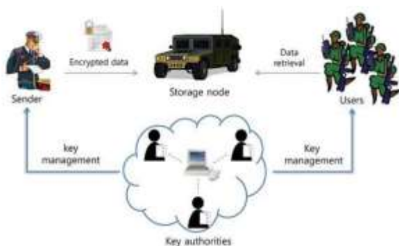
Figure. 1. Architecture of secure data retrieval using CP-ABE in a disruption-tolerant military network.
