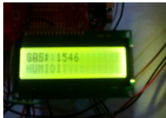
Fig: Gas and humidity displayed on LCD
