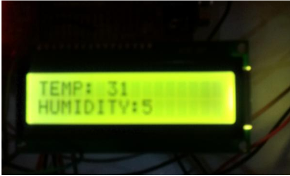
Fig: Temperature and humidity displayed on LCD.
