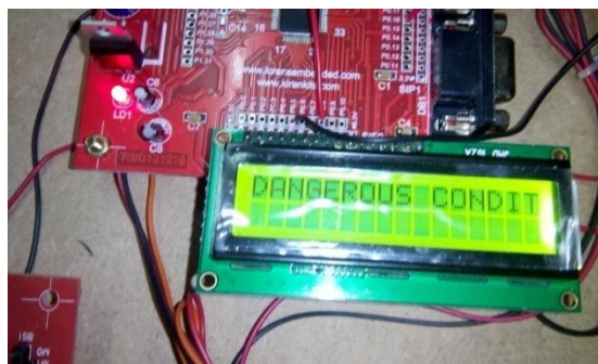
Fig .3 MEMS value is more then display dangerous condition on LCD.
