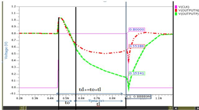
Fig. 2. Transient simulations of the conventional single-tail dynamic comparator at  $V_{cm} = 0.7$  V, and  $V_{DD} = 0.8$  V.
