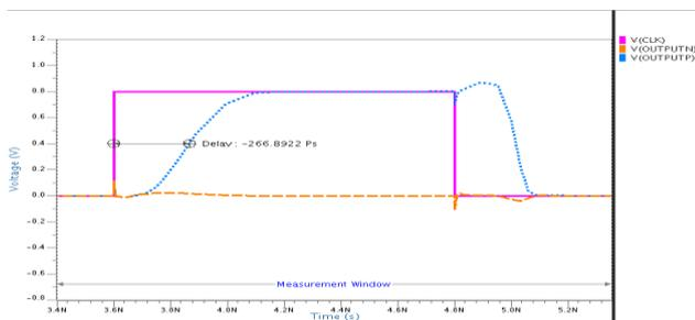
Fig.6. Transient simulations of the proposed double-tail dynamic comparator for  $V_{DD} = 0.8 V$ .
