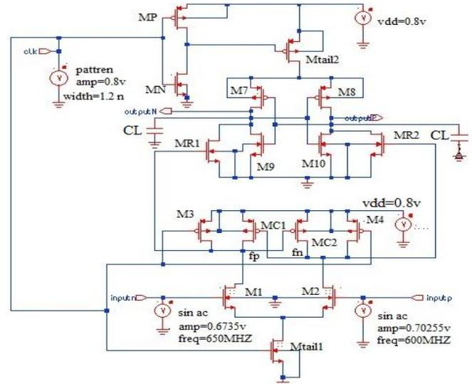
Fig.5. Schematic diagram of the proposed dynamic comparator.
