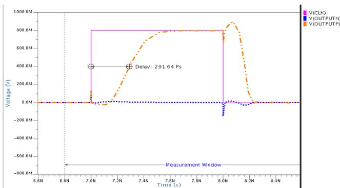
Fig. 4. Transient simulations of the conventional double-tail dynamic comparator for input voltage difference of  $V_{cm} = 0.7$  V, and  $V_{DD} = 0.8$  V.
