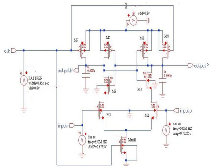
Fig. 1. Schematic diagram of the conventional single-tail dynamic comparator
