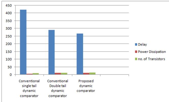
Fig.8.Comparison of Dynamic comparator Architectures
