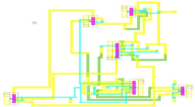
Fig.7. Layout of the proposed double-tail dynamic comparator
