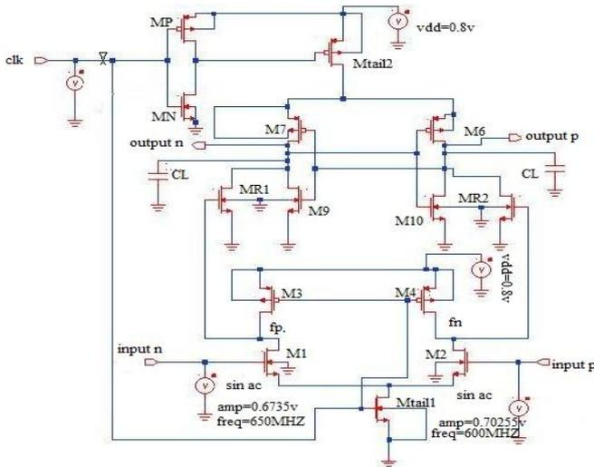
Fig.3. Schematic diagram of the conventional double-tail dynamic comparator
