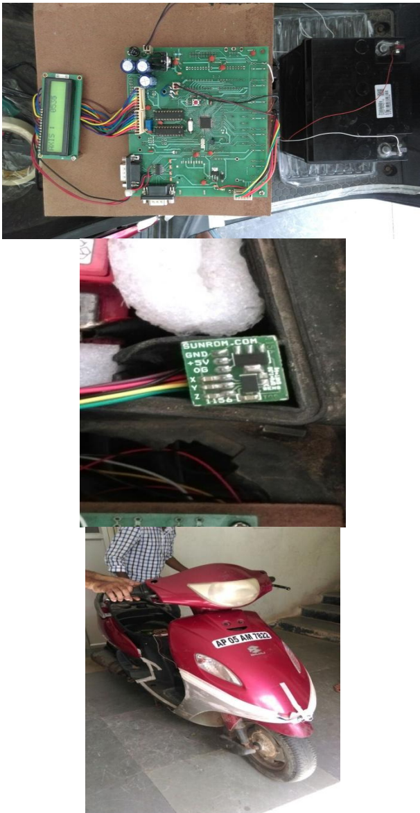
Figure 5.5 Crash prediction using ultrasonic sensor and Accelerometer
