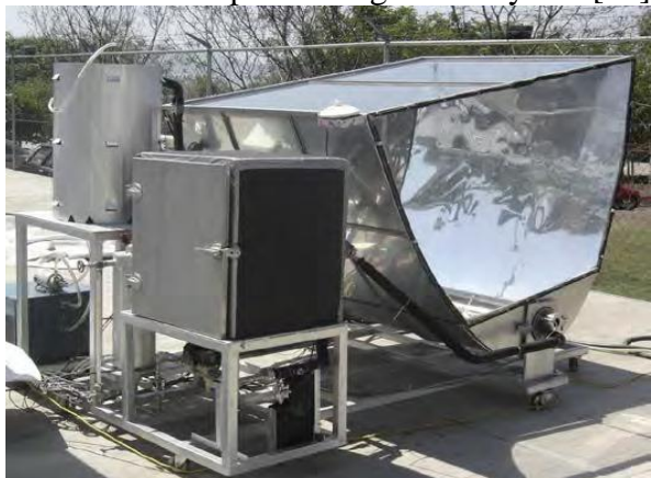
Fig. 3. Photograph of the solar intermittent absorption refrigeration system developed [21]
