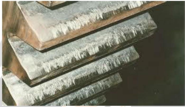
Fig.5 Gear scuffing Effect
