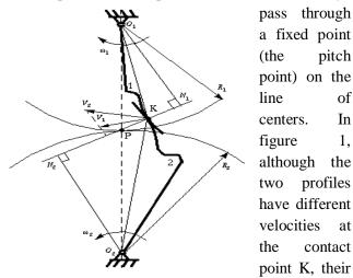
velocities along N1N2 that is passing through the pitch point P are equal in both magnitude and direction. Otherwise the two tooth profiles would separate from each other. Therefore, we get the velocity ratio, which is equal to the inverse ratio of the diameters of these two tooth profiles. This is called fundamental law of gear-tooth action. For each two mating gearing tooth profiles, they should satisfy the fundamental law to get a constant velocity ratio.
