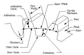
Usually we use the involute curve to generate a spur gear . The involute has important advantages -- it is easy to manufacture and the center distance between a pair of involute gears can be varied without changing the velocity ratio. Thus, we generate the involute curve to generate a spur gear
