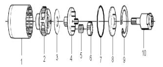
The gearbox focused on, and used for model validation in this report is a 2 stage planetary gearbox made by Atlas Copco. The exploded view shows the components of the gearbox that will be explained in this chapter.
