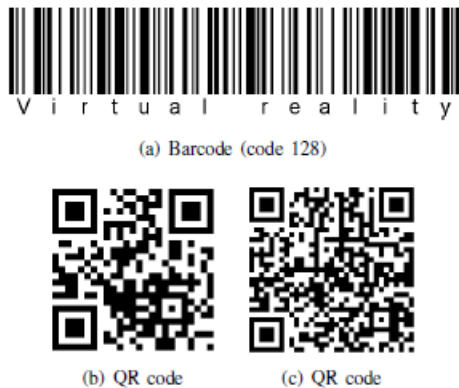
Fig. 1. Three different barcodes encoding the statement “Virtual reality”. (a) is a linear barcode (code 128), and (b) and (c) are matrix barcodes (of the QR code standard). While (b) encodes the plain text, (c) encodes an encrypted version using the AES-256 encryption algorithm in the cipher-block chaining (CBC) mode (note this last code requires a password for decryption).
