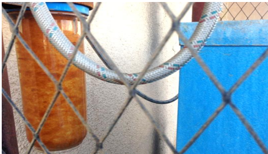
Fig. (2). The filter of a street cooler accommodating a variety of impurities and contaminants.
