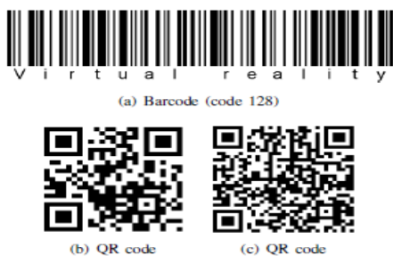
Fig. 1. Three different barcodes encoding the statement "Virtual reality". (a) is a linear barcode (code 128), and (b) and (c) are matrix barcodes (of the QR code standard). While (b) encodes the plain text, (c) encodes an encrypted version using the AES-256 encryption algorithm in the cipher-block chaining (CBC) mode (note this last code requires a password for decryption).
