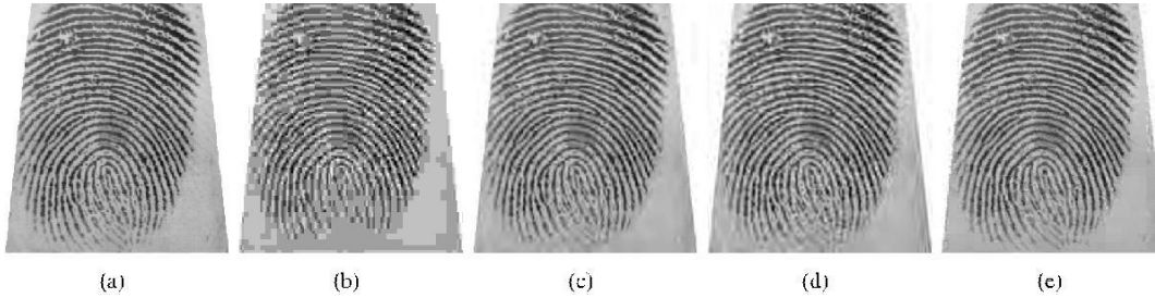
Fig. 14. (a) Original image with size 328 \times 364 , (b) JPEG, (c) JPEG 2000, (d) WSQ, (e) the proposed method at compression ratios 40 : 1.
