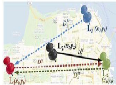
Fig. 2. PPFRVP scenario, where the fairness function is g = \text{argmin}_i (D_i^M) . The dashed arrows represent the maximum distance D_i^M from each user u_i to any user j \neq i , whereas the solid line is the minimum of all such maximum distances. The fair rendez-vous location is L_{fair} = L_2 = (x_2, y_2) .
