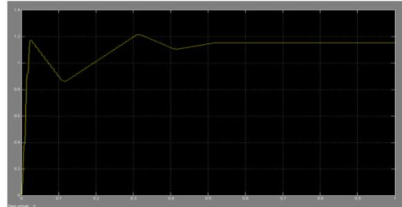
**Fig.4 The RMS voltage at AC buses under normal operation ,Generator bus**
