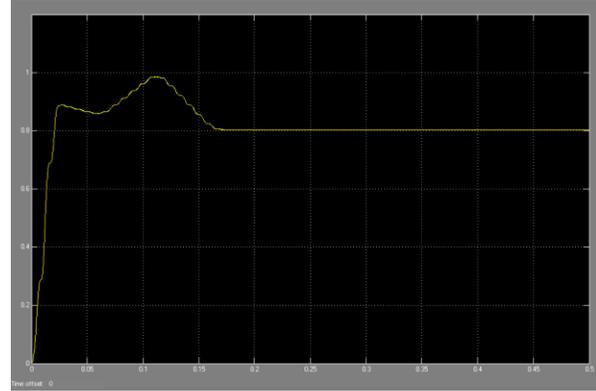
**Fig 18b The RMS current at load bus under short circuit (SC) fault condition at bus V**
