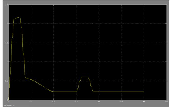
**Fig 20b The RMS current waveform at the load bus under load excursions**
