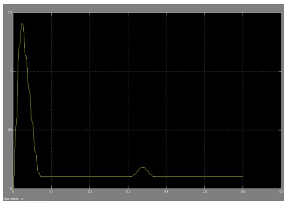
**Fig 20a The RMS current waveform at the load bus under load excursions**
