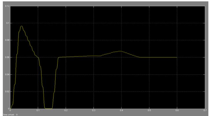
**Fig 21a The linear load RMS current waveforms**
