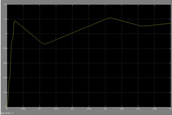
**Fig 17a The RMS voltage at generator bus under short circuit (SC) fault condition at bus V**
