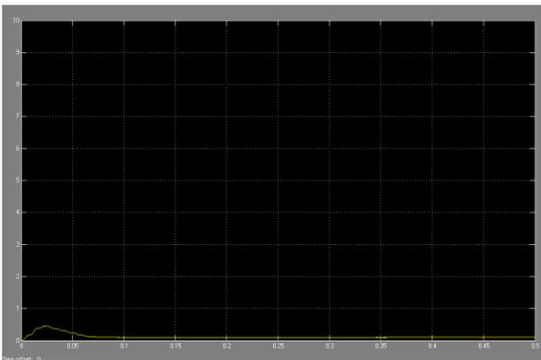
**Fig 18a The RMS current at generator bus under short circuit (SC) fault condition at bus V**
