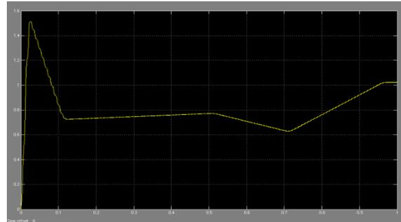
**Fig 8b** The RMS current at the infinite bus under normal operation
