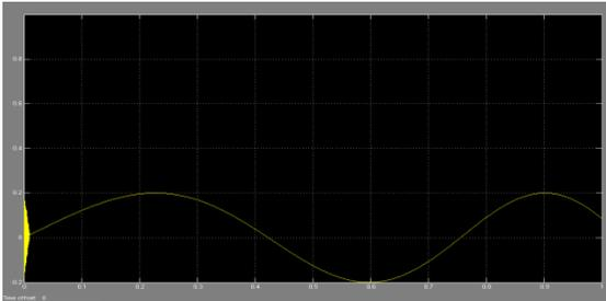
**Fig 6a**The reactive power at AC buses under normal operation ,Generator Bus
