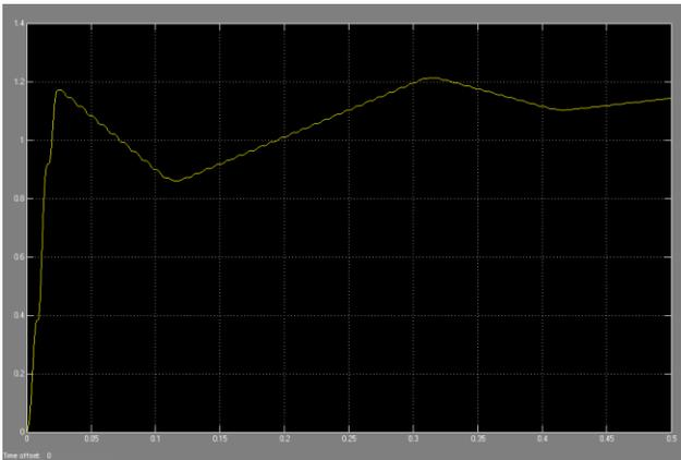
**Fig 17b The RMS voltage at load bus under short circuit (SC) fault condition at bus V**
