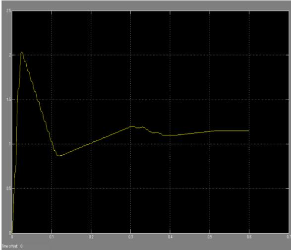
**Fig 19a The RMS voltage waveform at the generator bus under load excursions**
