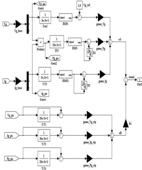
**Fig. 2b MATLAB functional model of the Inter-coupled tri loop error driven modified PID controller**
