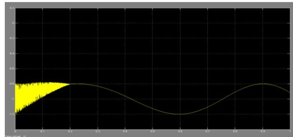
**Fig 9a** The reactive power at the infinite bus under normal operation
