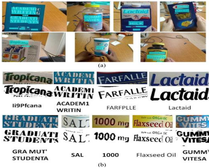
Fig. 16. (a) Some results of text localization on the user-captured dataset, where localized text regions are marked in blue. (b) Two groups of enlarged text regions, binarized text regions, and word recognition results from top to down.
