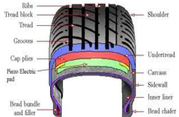
Fig-2 Piezoelectric tire installed with pad
