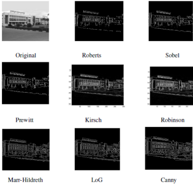
Figure: 4 Original Image with the result of various edge detection techniques.
