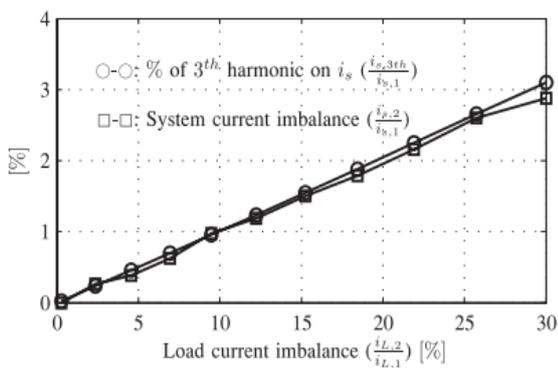
Fig. 4. Relationship between permissible unbalance load currents, the corresponding third-order harmonic content, and system current imbalance (with respect to positive sequence of the system current,  $i_{s,1}$ )
