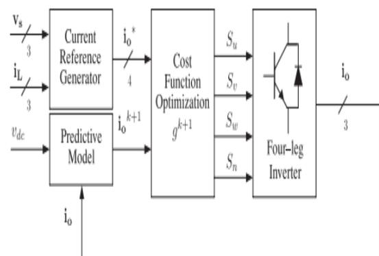
Fig. 2. Proposed predictive digital current control block diagram
