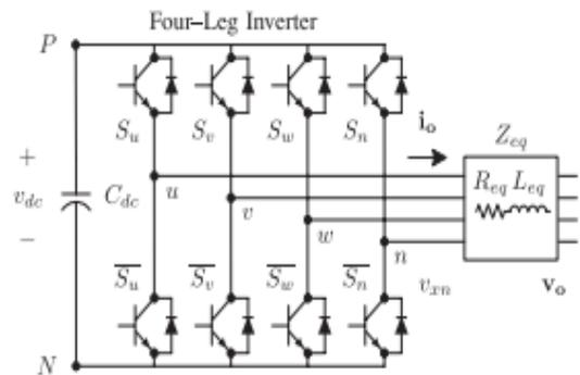
Fig. 1. Two-level four-leg PWM-VSI topology
