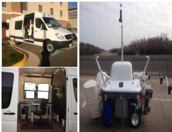
Fig .1. The bridge robotic inspection system with the command center built in the transportation van. the IE and USW data collection and analysis. Finally, we provide conclusions from the
