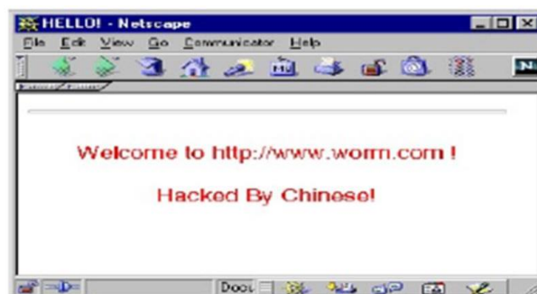
Fig- 6 The Code Red worm, also called Bady, was the first widespread pure worm in the modern Internet. It spreads using web-servers and may modify the contents of the server.
