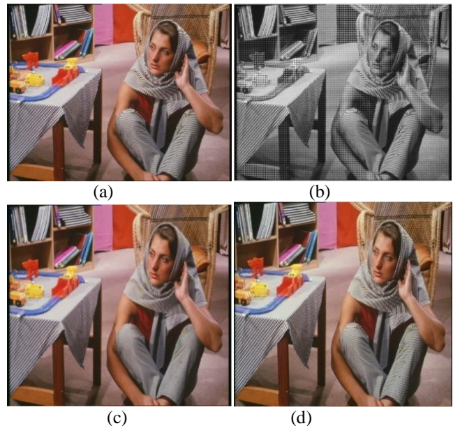
Result1 (a) input image (b) bayer pattern genetration of input image (c) Demosaicing using bilinear (d) original image by content based color correlation analysis
