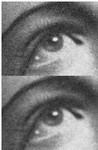
Figure 2 Gaussian blur can be used in order to obtain a smooth grayscale digital image.
