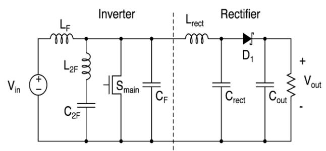
Fig 1. Very High Frequency Resonant Boost Dc-Dc converter.
