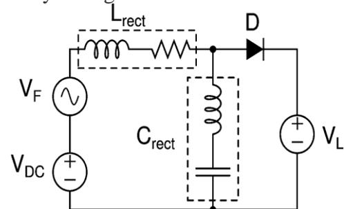
Fig. 2. Schematic of rectifier is implemented in the Matlab for designing purpose.
