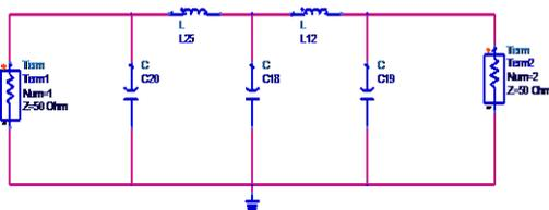
fig.1. Chebyshev Filter Schematic Design
