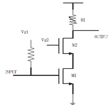
fig.2. Schematic of cascaded LNA
