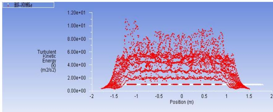
Fig-3.2 Turbulent Kinetic energy for cylinder with vortex generator (delta) flow from wedge side
