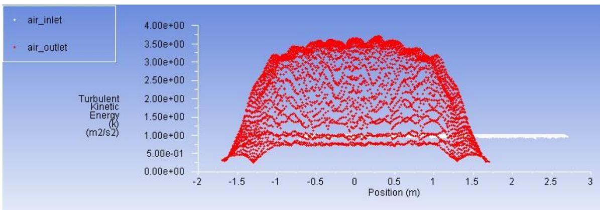
Fig-3.4 Turbulent Kinetic energy for cylinder with vortex generator (dent) side.
