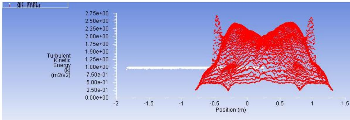
Fig3.8 Turbulent Kinetic energy graph for bent cylinder with vortex generator (dent).
