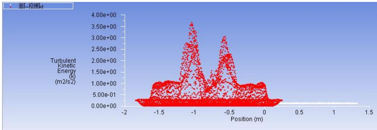
Fig3.7 Turbulent Kinetic energy graph for bent cylinder with vortex generator (delta) flow from ramp side.
