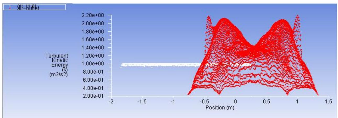
Fig3.6 Turbulent Kinetic energy graph for bent cylinder with vortex (delta) flow from wedge side
