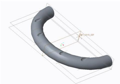
Fig 2.4 Bent Pipe with dent type vg
