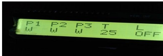
Fig no 6 Soil sensor status in presence of water in soil.
